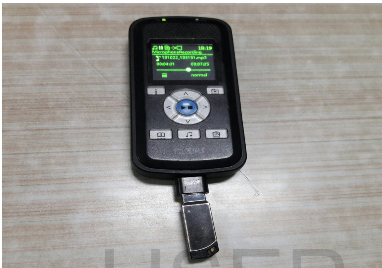
Figure 5: A DAISY player that is used for navigating visually impaired learners for accessing something as complex as an encyclopedia or textbook
